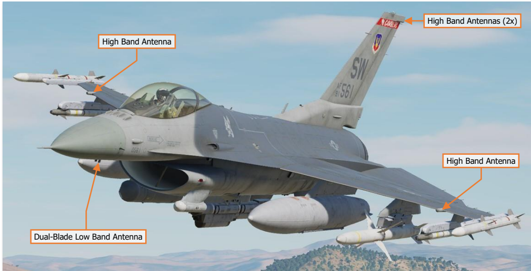
AN/ALR-56M Advanced RWR Antenna Locations
