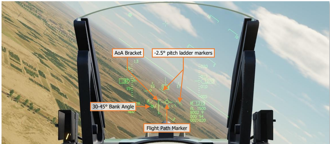
AoA and glide path references in base turn to final
