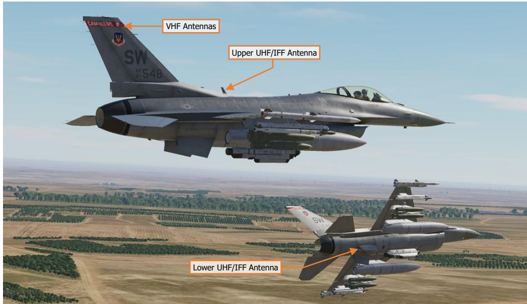
AN/ARC-164 & AN/ARC-222 Radio Antenna Locations
