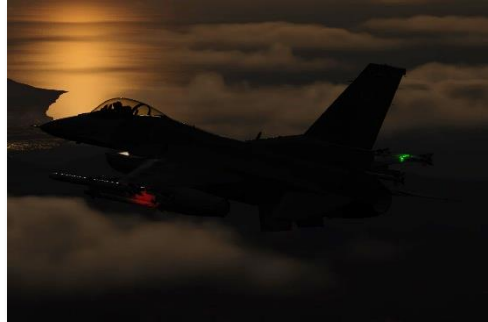
All lights off except FORM knob; FORM knob set to minimum
