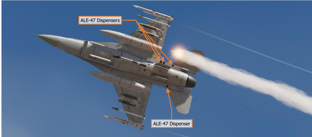
AN/ALE-47 Airborne Countermeasures Dispenser Locations
